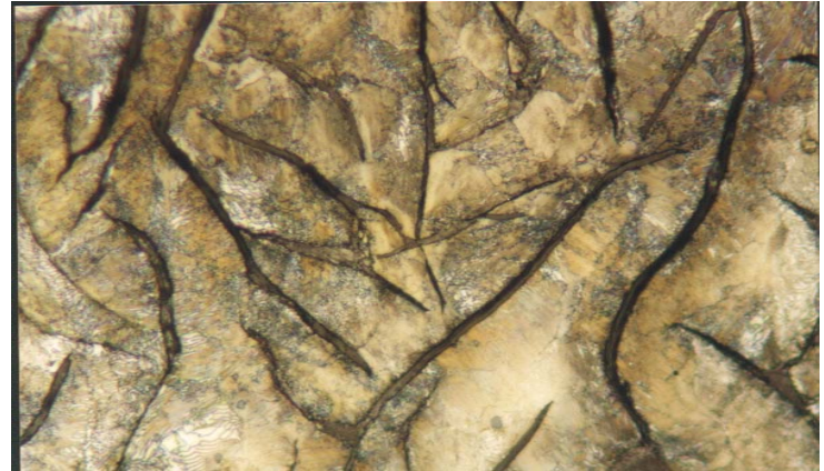
Gray Cast Iron, Brightfield Magnification: 550X Etching: 2% Nital
